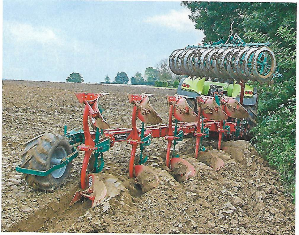
The packer can be raised up out of work when turning the furrows to the right. This allows easy and convenient working up to a headland or obstacles ... to minimise the unploughed area.
