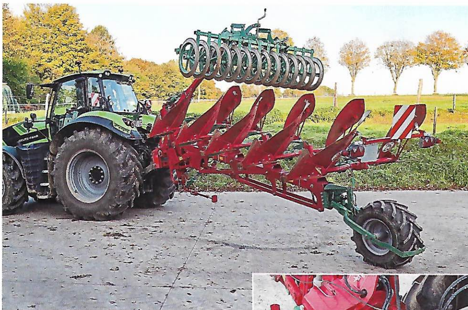
In transport, the rear depth wheel is fixed with the plough pivoting at the headstock. The combination handled like a single-wheeled trailer and 'rode' well.
