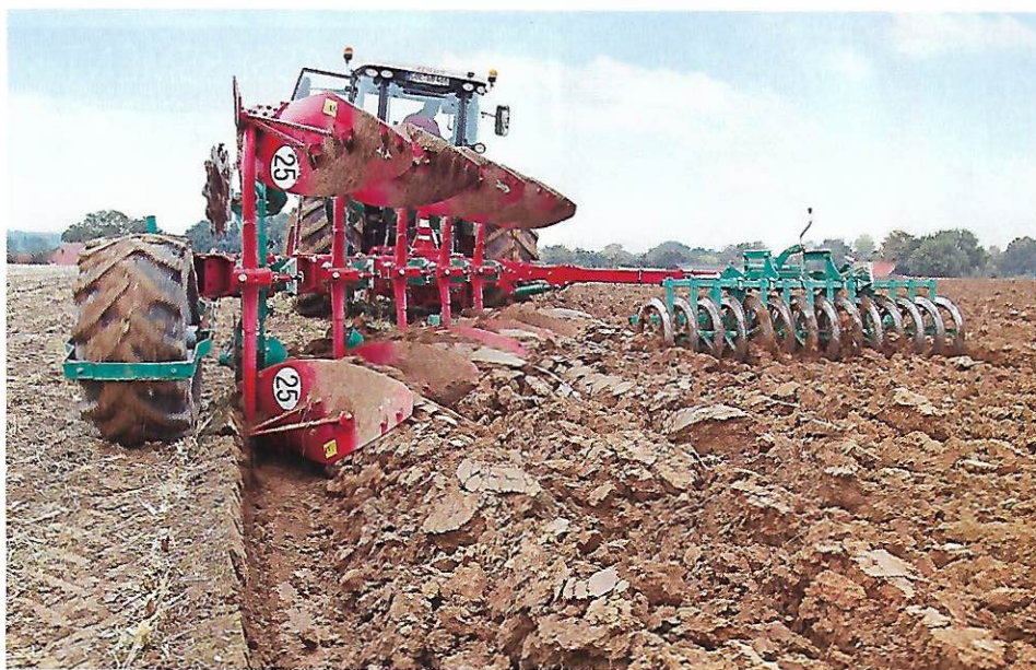
The No. 38 bodies cleared the furrow bottom cleanly and delivered a good quality of work. When set to a maximum furrow width of 455mm, the bodies could work to a depth of 300mm.
