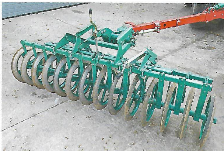
The load on the Packomat and its accompanying harrow is adjusted via a mechanical screw handle (above, left). The packer is raised and swivelled by two cylinders (above, right). The turnbuckle in the right photo is used to align the packer rings and indirectly to influence the line of draft.
