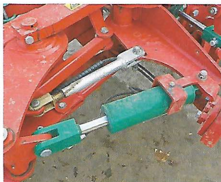
Turnbuckle to one side sets plough alignment.
