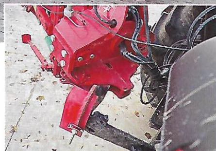
In transport, the rear depth wheel is fixed with the plough pivoting at the headstock. The combination handled like a single-wheeled trailer and 'rode' well.
